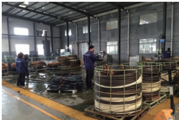
Static Pressure Testing
